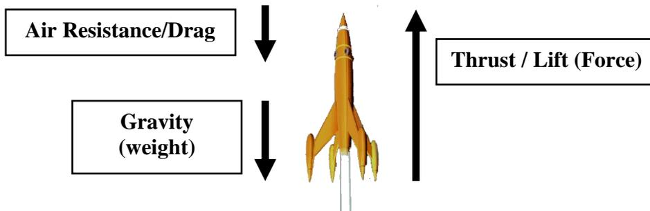
Newton's Laws of Motion help to explain a rocket in flight. First law states that rockets will stay in motion until acted on by an outside force (this is Inertia). The outside forces acting on your rocket are gravity and air resistance. If your rocket was able to reach the escape velocity on Earth (~25,000 mph) it would keep traveling forever in space (unless it hit a planet, asteroid or entered another gravitational field)
